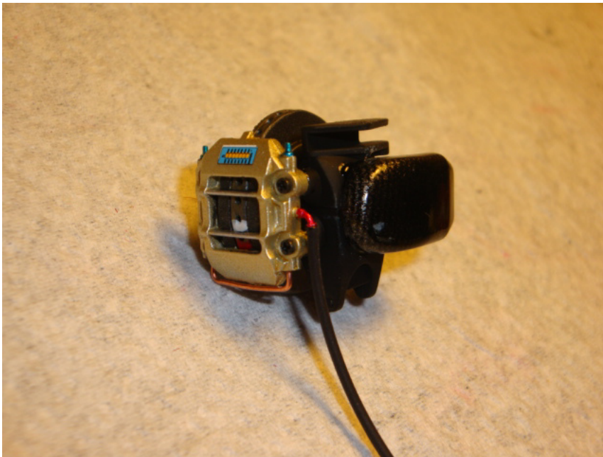
Left front brake assembly with connection pipe to the braking system
