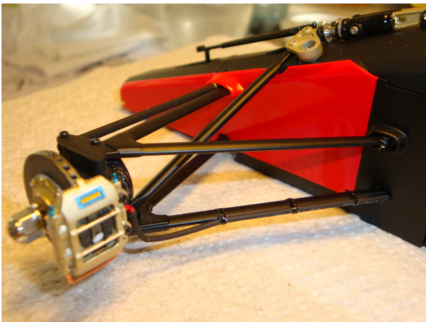
Left front brake assembly mounted on the chassis and connection to the braking system
