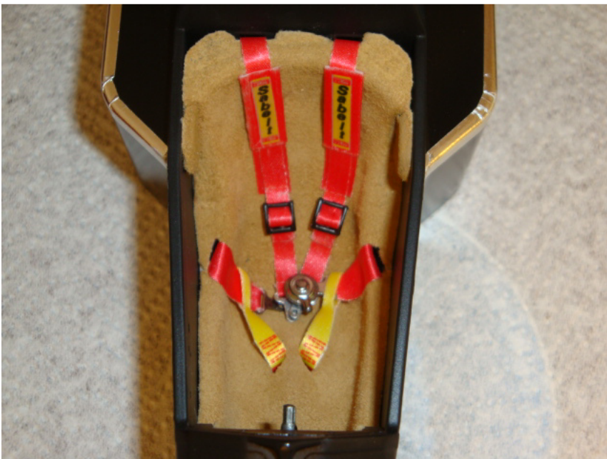
Seat with seat belts, installed in the chassis
